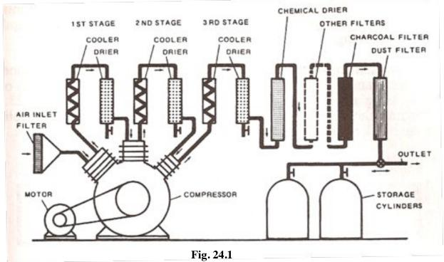
Schematic diagram of a compressor system with filters.
