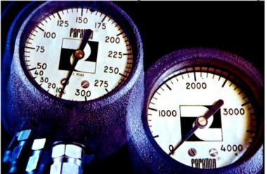
"Reserve" valves are not adequate substitutes for contents gauges since they may be inadvertently opened before or during the dive, and have been observed to leak or fail under operational conditions.
