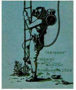
The development of **self-contained** air supplies was impeded by the lack of sufficiently powerful compressors and reservoirs. In 1863 the Frenchmen, Rouquayrol and Denayrouze, invented the first satisfactory demand regulator for self-contained underwater breathing apparatus (SCUBA), but due to lack of suitable high pressure air compressors and cylinders, it was limited to surface air supply lines.
