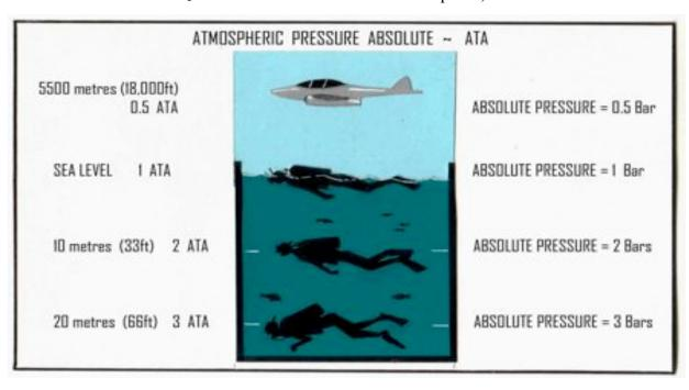
Fig. 2.2 Atmospheric and Hydrostatic Pressures (depth) added and thus converted to Absolute Pressure
