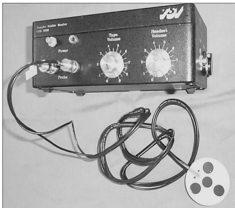
Figure 4-24. Doppler bubble monitor showing transmitting and receiving probe.
