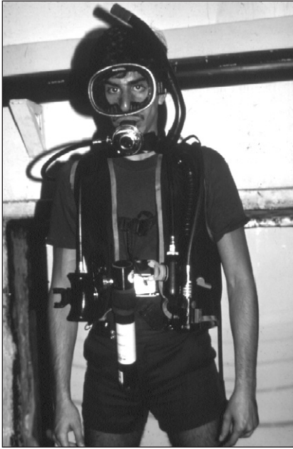
Figure 17-4. A diver wearing several alternative air sources. From right: a secondary regulator attached to the first stage (Octopus), a small cylinder of compressed air (SpareAir), a regulator attached to a buoyancy compensator, and a spare regulator attached to a second compressed air tank (pony bottle). (Photograph courtesy of Glen H. Egstrom.)
