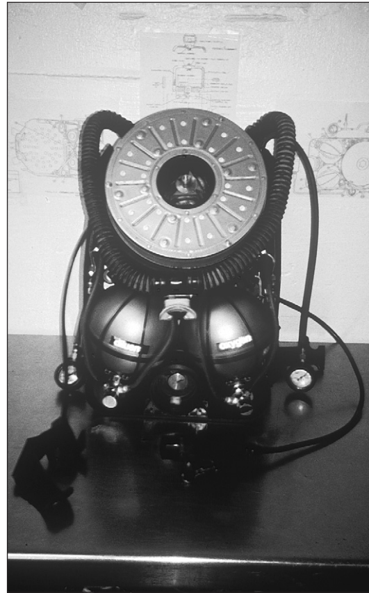
Figure 3-7. Closed-circuit rebreathing device showing counterlung and gas supply. (Photograph courtesy of Lee Somers.)
