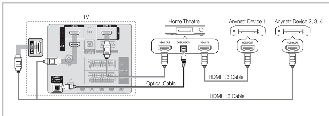
1. Connect the **HDMI IN (1(DVI), 2, 3 or 4)** jack on the TV and the **HDMI OUT** jack of the corresponding Anynet+ device using an HDMI cable.
