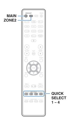
Settings such as the input source, volume level and sound mode can be registered to the QUICK SELECT 1 - 4 buttons.
