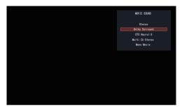
This unit provides not only sound modes that conform to the formats recorded on discs such as Dolby and DTS, but also extended types of modes that match your speaker configuration and "original sound modes" that create atmosphere of Rock Arena and Jazz Club, etc.
