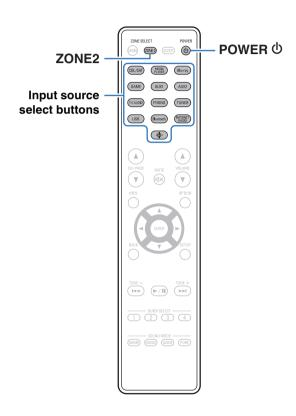
1 Press ZONE2 to set the operating zone to ZONE2 with the remote control.
